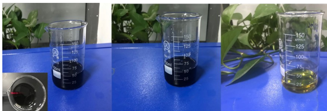
Fig. S6. The stability test for d-V 4 C 3 T x MXene nanosheets at room temperature.
