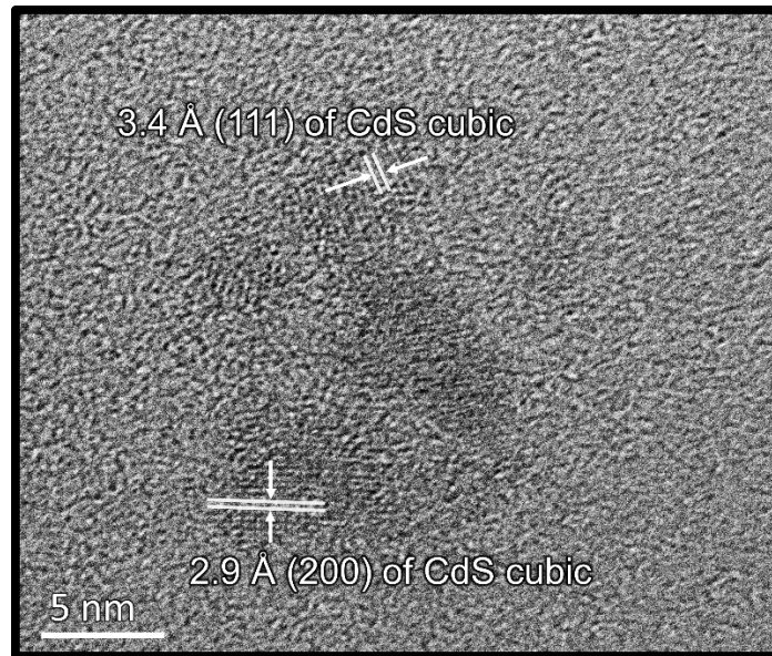
Fig. S6 TEM image of CdS nanoparticle with the (111), (200) lattice fringe of CdS cubic structure.
