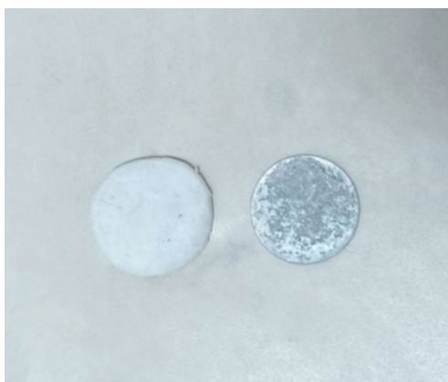
Fig. S2. Optical image of Zn anode based on ZS electrolyte after cycling at 5 \text{ mA cm}^{-2} , 5 \text{ mA h cm}^{-2} .
