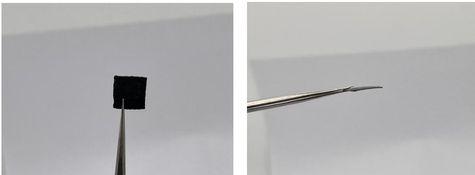
Fig. S1 Post-pressing: Electrode materials loaded on nickel foam.
