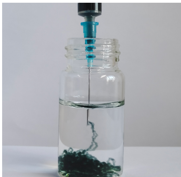
Fig. S8 Digital photograph of the injectability of the pAMPS-Cl/AuNR@HA-DA hydrogel.
