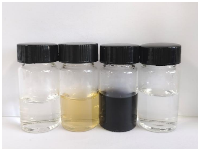
Fig. S7 Photograph of the color change of pAMPS-Cl during the iodometric assay.
