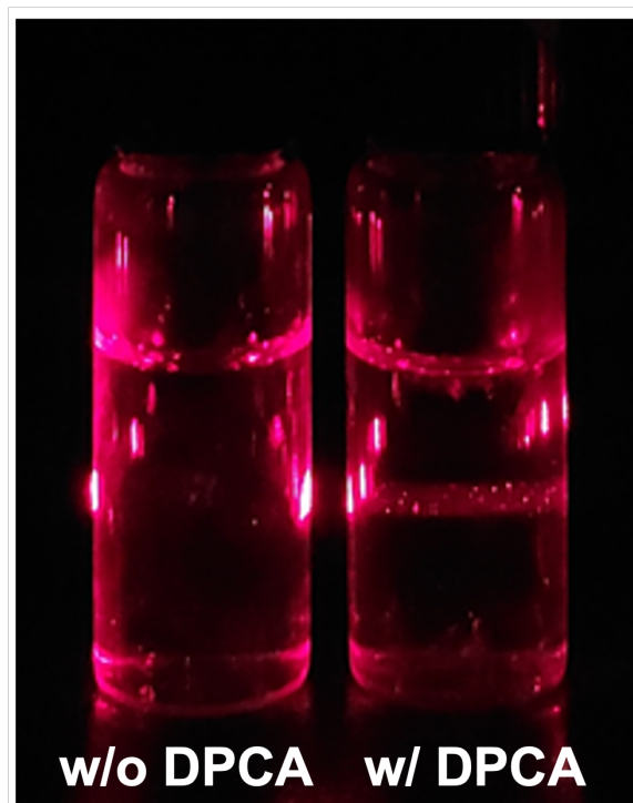
Fig. S3. Optical image demonstrating the Tyndall effect exhibited in the solution containing 1,4-DPCA aggregates.
