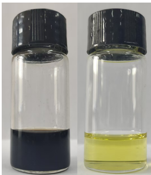
Figure S1. Digital photographs showing raw product in the presence (left) and absence (right) of the Cu salt in the cluster synthesis.
