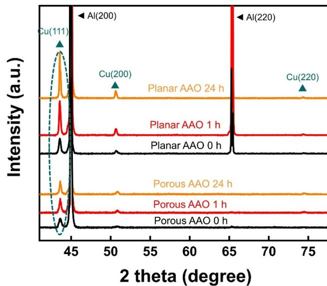
**Figure S4.** XRD patterns of the Cu seeds deposited on the porous and planar AAO after annealing at 250 °C for 0, 1, and 24 hours.
