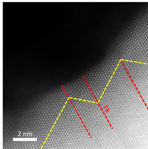
**Figure S2.** Dark-field scanning transmission electron microscopy (DF-STEM) micrograph revealing the atomic-resolution image of the twin structure in the nt-Cu nanowire.
