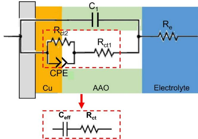
**Figure S5.** The equivalent circuit model for the porous AAO-templated electrode in an electrochemical cell.
