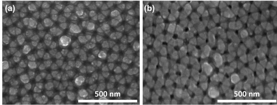
**Figure S3.** Planar SEM image of the Cu seed deposited on the porous AAO template before and after annealing at 250 °C for 1 hour.
