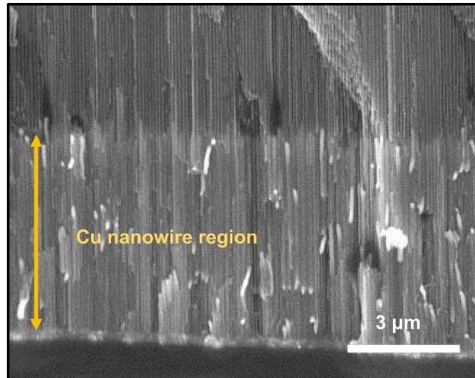
**Figure S1.** Cross-sectional SEM image of the AAO template with electrodeposited nt-Cu nanowires.
