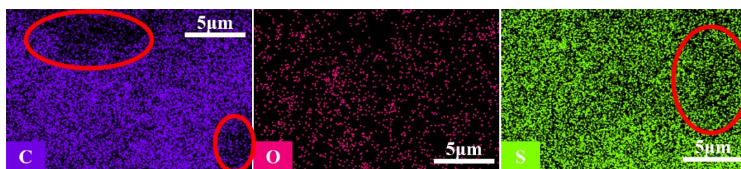
Fig. S3 EDS mapping of C, O and S elements in the cathodes of PVDF-based Li-S batteries.
