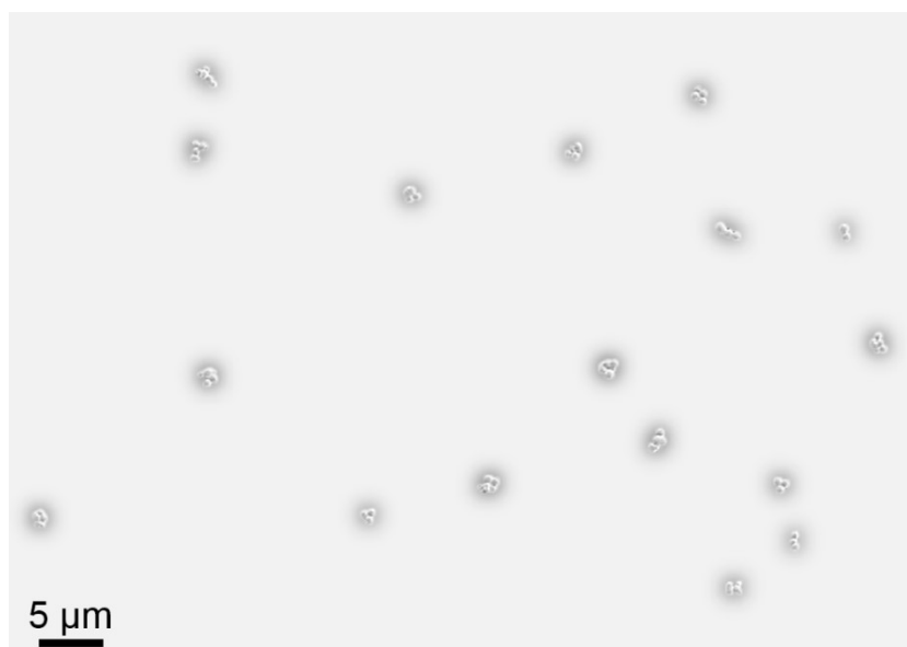
Figure S4. SEM images of the colloidal clusters with \langle N \rangle = 4.2 . The colloidal clusters were obtained by first adding an appropriate amount of ethanol (4.2 mL) into the THF solution of IAC-4 (2.0 mg/mL, 1 mL) with the adding rate of 86.4 mL/h and meanwhile the dispersion was stirred with a rate of 1800 rpm. After adding ethanol, the stirring was continued for 15 min with the stirring rate of 1500 rpm. Finally, 20 mL ethanol was quickly added into the dispersion to quench the structures. The dispersions were placed for 3 days before fabricating samples for SEM observations.
