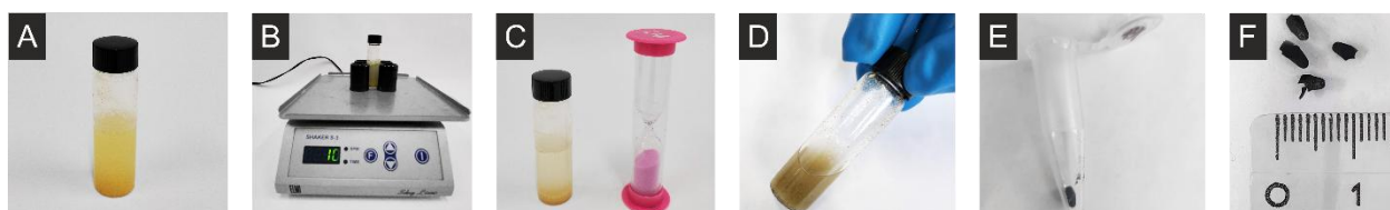
Figure S1. Preparation procedure for Pd/ P. yeei catalyst: A – mixture of bacterial cells with palladium acetate, B – 10 minutes of shaking, C – reduction of Pd(II) to Pd(0), D – mixture of cells with Pd nanoparticles, E – harvested catalyst in test tubes, F – dried Pd/ P. yeei catalyst
