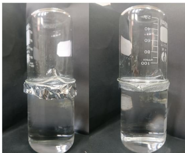
Fig. S9. Water vapor transmission: aluminum foil (left) and cling film (right).
