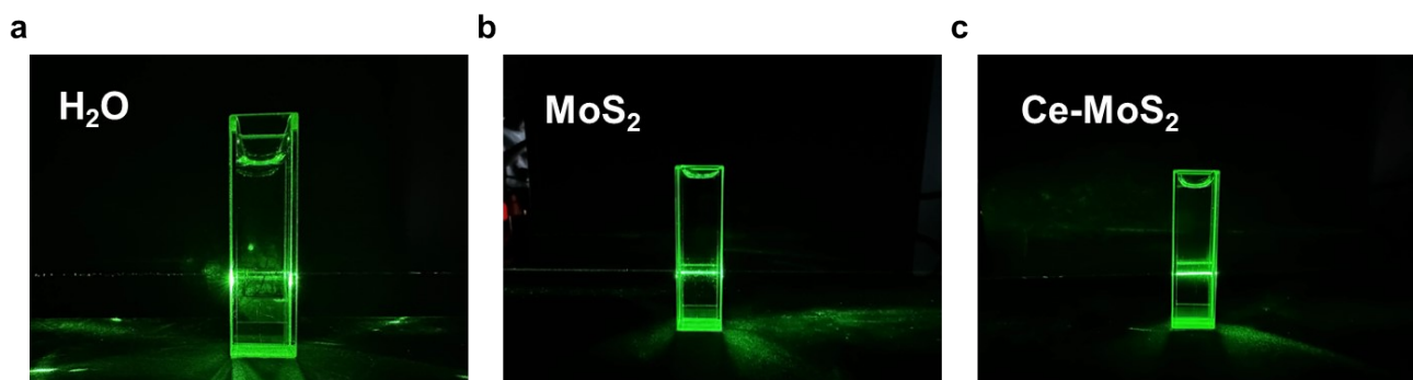
Fig. S1. Unique Tyndall effect for (a) water, (b) MoS_2 clusters and (c) Ce-MoS_2 clusters under 532 nm excitation.
