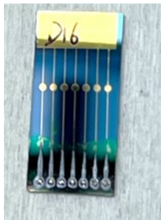
Figure S6. Photograph of selective deposition of PbSe QDs onto conductive gold traces on Si/SiO 2 . Gold traces have a linewidth of 100 \mu m and a circle at the bottom of the traces of 1mm in diameter. Small amount of PbSe on non conductive area is from dip-coating effect.
