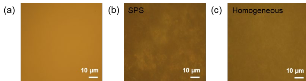
Figure S11. The OM image of (a) homogeneous solution, (b) after adding EA to generate SPS and (c) after adding EA/ ethanol to generate homogeneous aggregation for GO/PEO.
