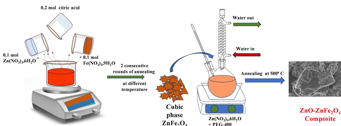
Fig. S 1. Schematic of synthesis procedure of ZnO-ZFO heterostructure.
