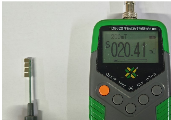
Fig. S7. The magnetic field strength of magnet used in in vitro simulation experiment.
