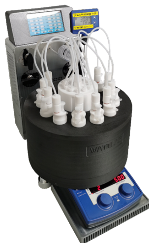
Figure S18: The picture of photocatalytic reactor. The photocatalytic reaction was performed on WATTCAS Parallel Photocatalytic Reactor (WP-TEC-LC) with 10W COB LED.
