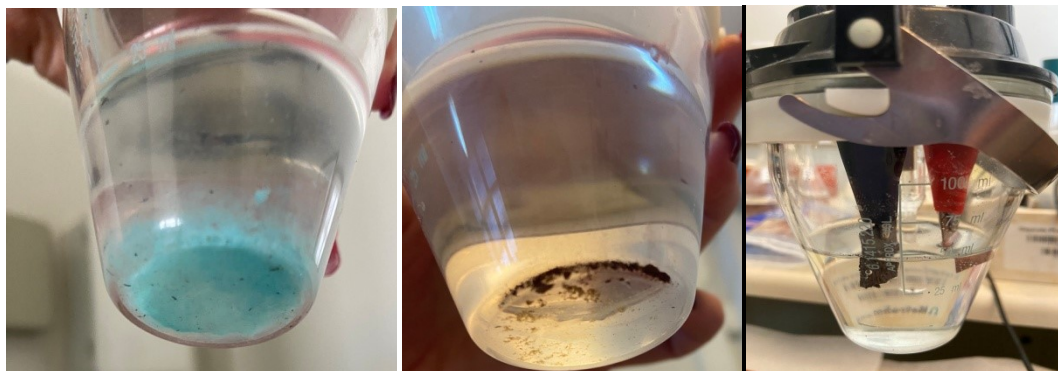
Fig. S3. Oxidation of the copper substrate (left), loss of material in the aqueous electrolyte (middle) due to electrolysis (right) on the surface of the bare \alpha - \text{Fe}_2\text{O}_3 electrode in \text{Li}_2\text{SO}_4 .
