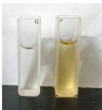
Fig. S12 Color changes of DMSO solution before and after BHCO and \text{Cu}^{2+} reaction.
