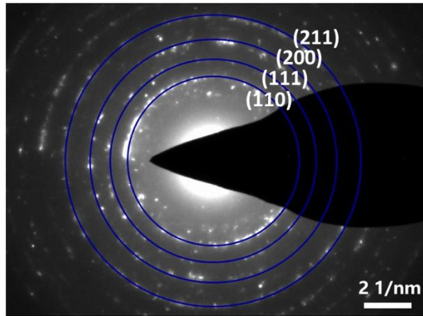
**Figure S4.** Selected area electron diffraction (SAED) pattern of a single LLTO nanowire.
