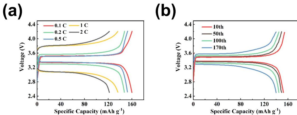
**Figure S13.** Charge/discharge curves of Li/PEO-VLSPE/LFP cell of (a) rate performances at 60 °C and (b) different cycles at 0.2 C and 60 °C.
