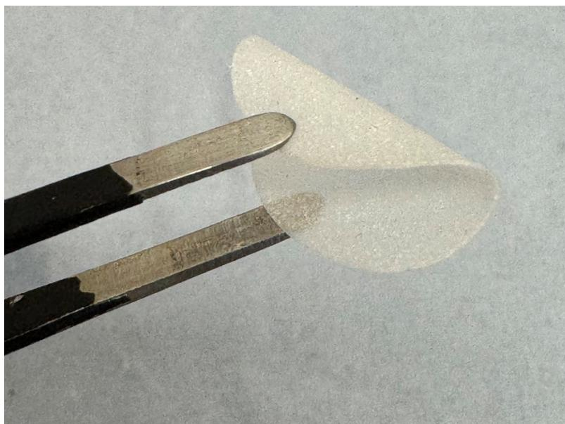
**Figure S14.** Digital photographs of VLSPE under mechanical bending.
