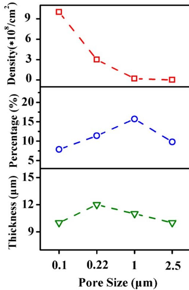
**Figure S2.** PC membranes' relationships of Pore Size vs Parameter: Diameter vs Thickness (PC membranes' thicknesses), Diameter vs Percentage (total pore area as a percentage of total membrane area) and Diameter vs Density (number of micro holes per square centimeter), respectively.
