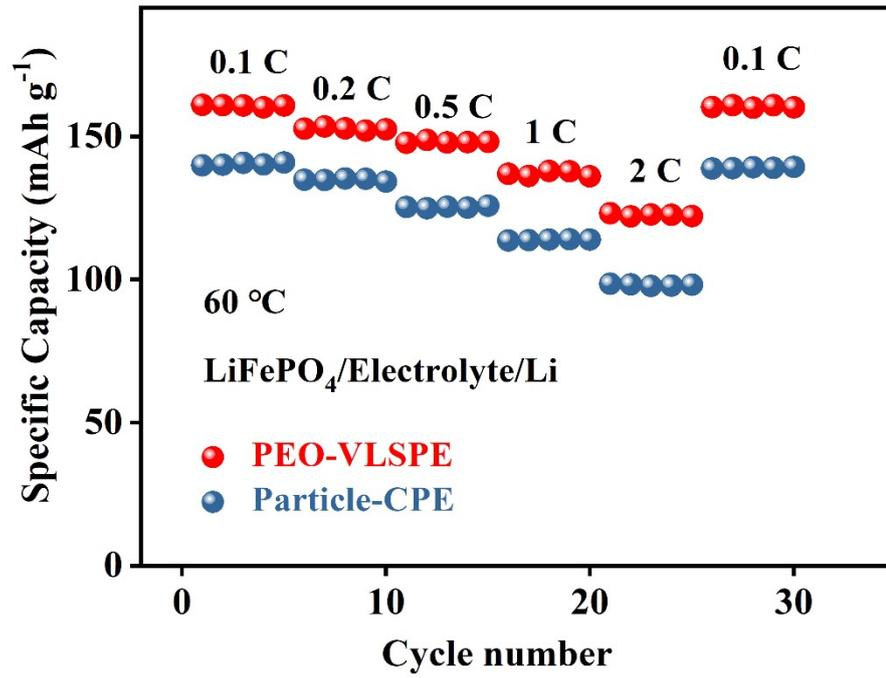
**Figure S11.** The rate performance curves between PEO-VLSPE and Particle-CPE.
