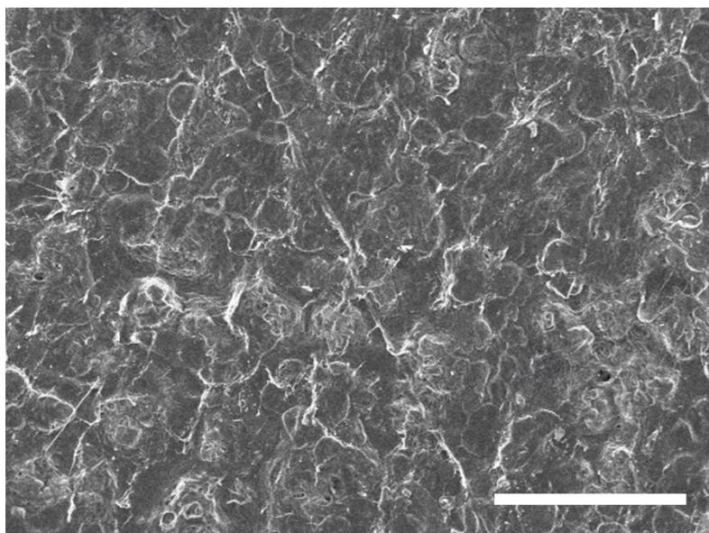
**Figure S16.** PEO-VLSPE after cycling. Scale bar, 10 $\mu$ m.
