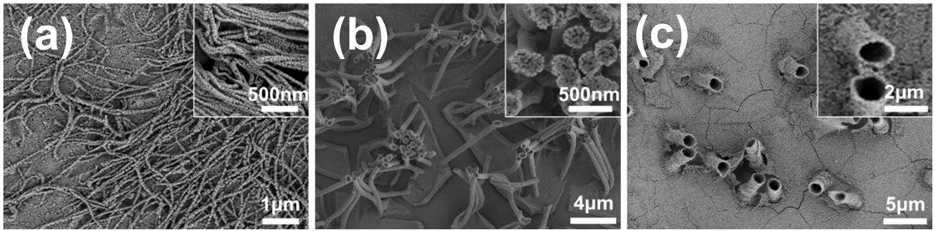
**Figure S3.** SEM images of VLNAs with different nano-array diameters: (a) 0.1  $\mu\text{m}$ , (b) 1  $\mu\text{m}$  and (c) 2.5  $\mu\text{m}$ , respectively.
