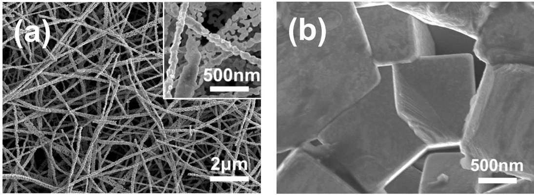
**Figure S10.** SEM images of (a) electrospun LLTO nanowires, (b) particle LLTO.
