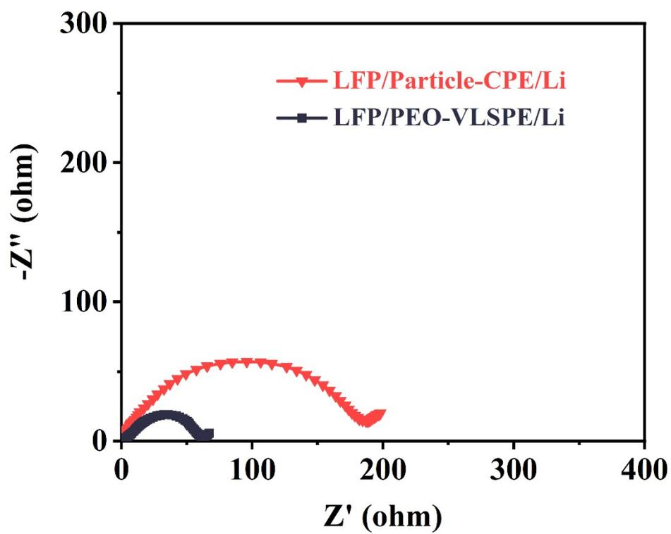
**Figure S12.** EIS of LFP/Particle-CPE/Li battery and LFP/PEO-VLSPE/Li battery.
