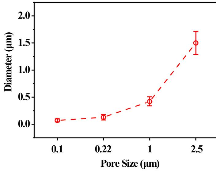
**Figure S8.** Diameter distribution of VLNA corresponding to PC templates with different pore sizes.
