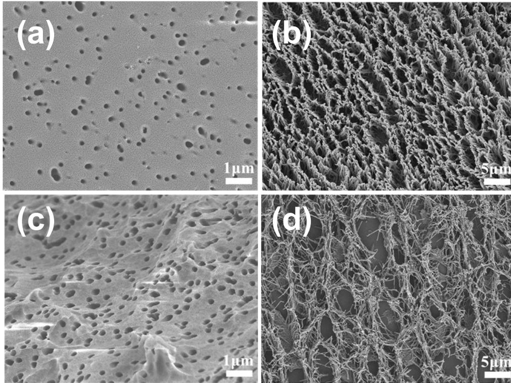
**Figure S9.** SEM images of flat and rough surfaces of PC templates and their corresponding VLNAs. (a) SEM image of PC-0.22 flat surface and corresponding (b) prepared VLNA, (c) SEM image of PC-0.22 rough surface and corresponding (d) prepared VLNA.
