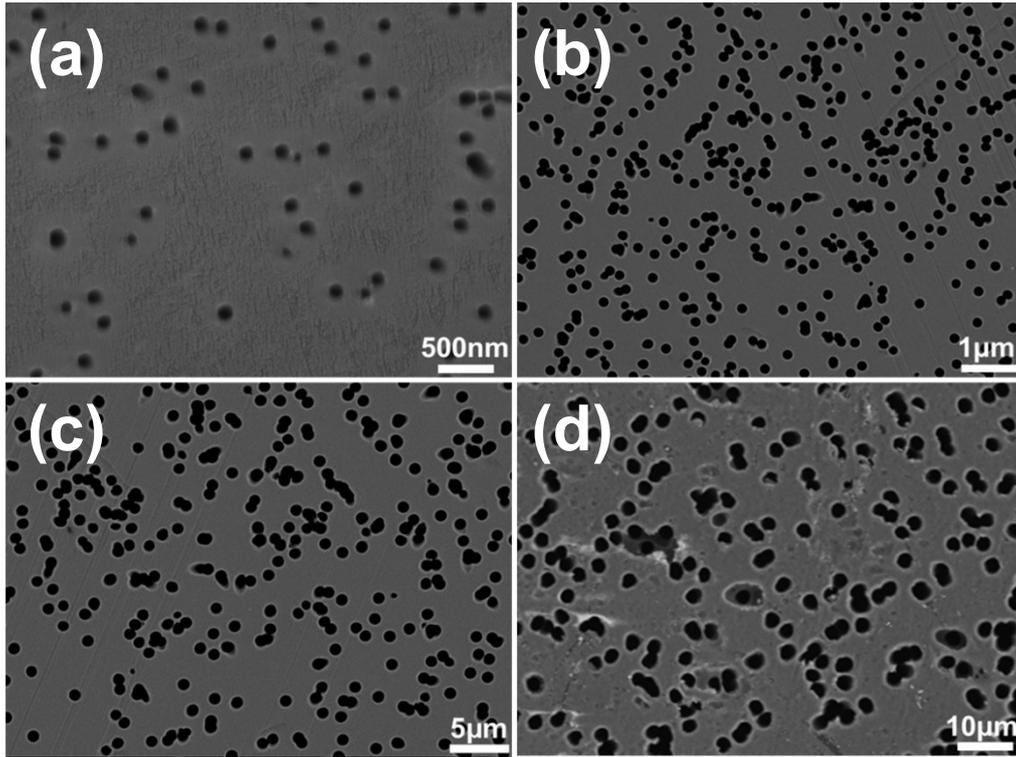
**Figure S1.** SEM images of flexible polycarbonate (PC) template: (a) PC-0.1, (b) PC-0.22, (c) PC-1, and (d) PC-2.5.
