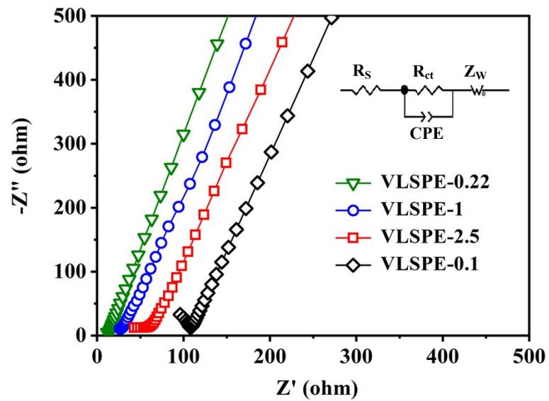
**Figure S7.** EIS curves for VLSPE with different pore diameters under 25 °C.
