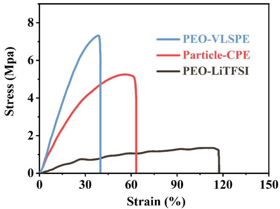
Figure S15. Stress-strain curves of composite electrolytes.
