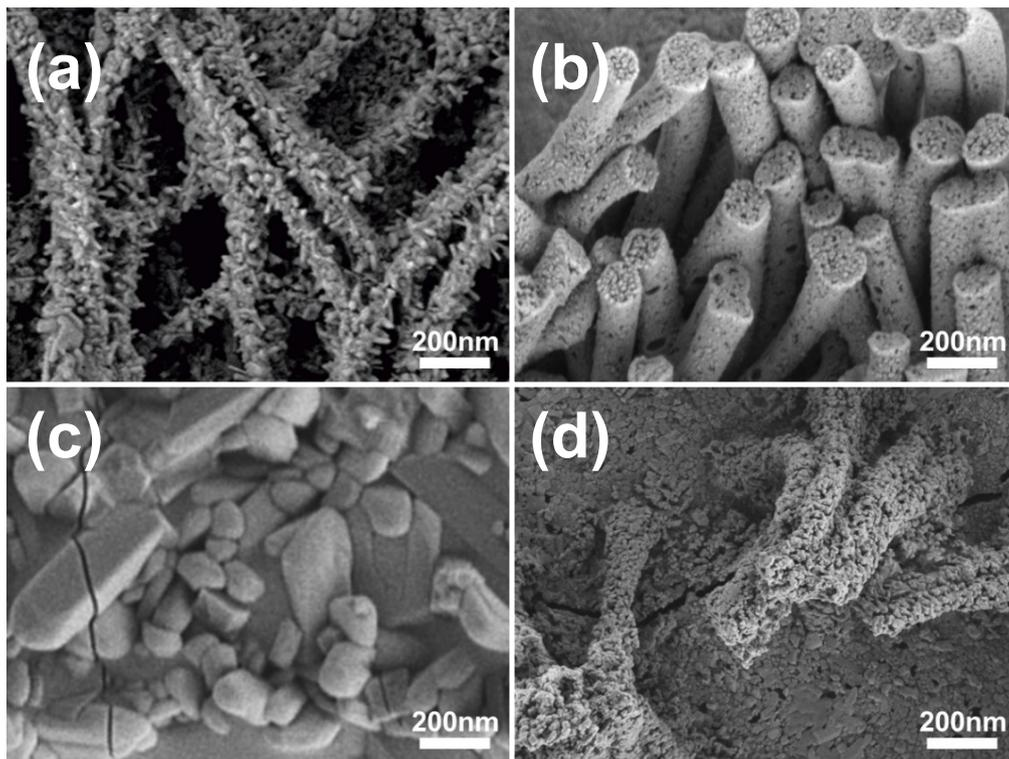
**Figure S5.** SEM images of VLSPE-0.22 at different heat treatment process: (a) 700 °C for 3 hours, (b) 800 °C for 3 hours, (c) 900 °C for 3 hours, and (d) 800 °C for 1 hour.
