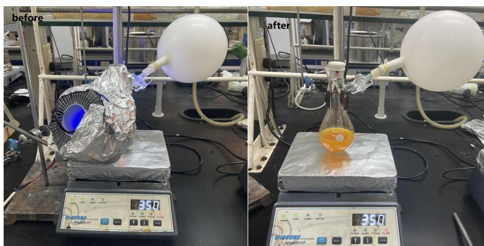
Figure S1. The setup for the blue LEDs-driven large-scale reaction
