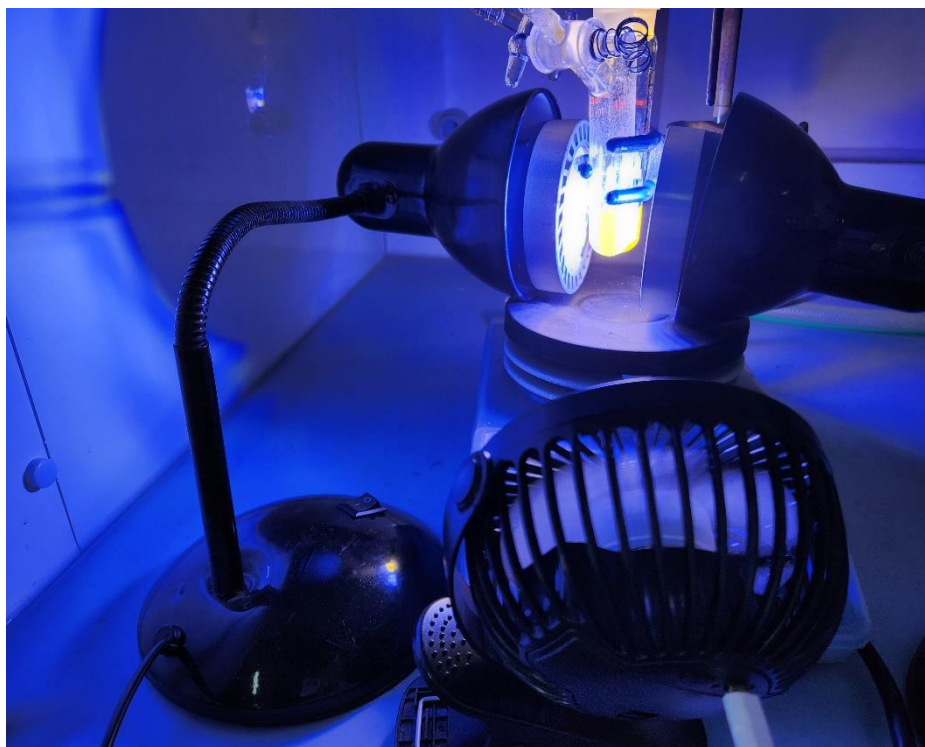
Figure S1. Typical experimental setup for photoredox catalytic reactions.
