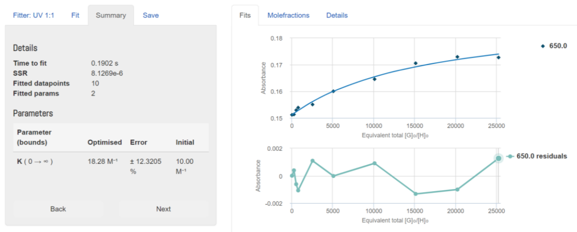
Figure S51: Least-squares nonlinear fitting of the normalized change in absorbance at 650 nm obtained as a function of concentration based on the UV-vis titration of 3 with D-mannose. The solid lines were obtained from nonlinear curve-fitting to a 1:1 binding model using the www.supramolecular.org web applet. ( http://app.supramolecular.org/bindfit/view/9347ed7b-bd0e-4954-9dbf-d3ce12bfc90 ).
