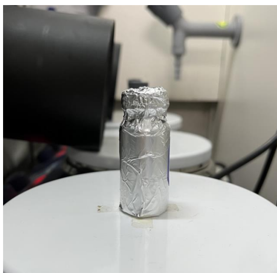
Fig S4 Setup for control reactions in dark
