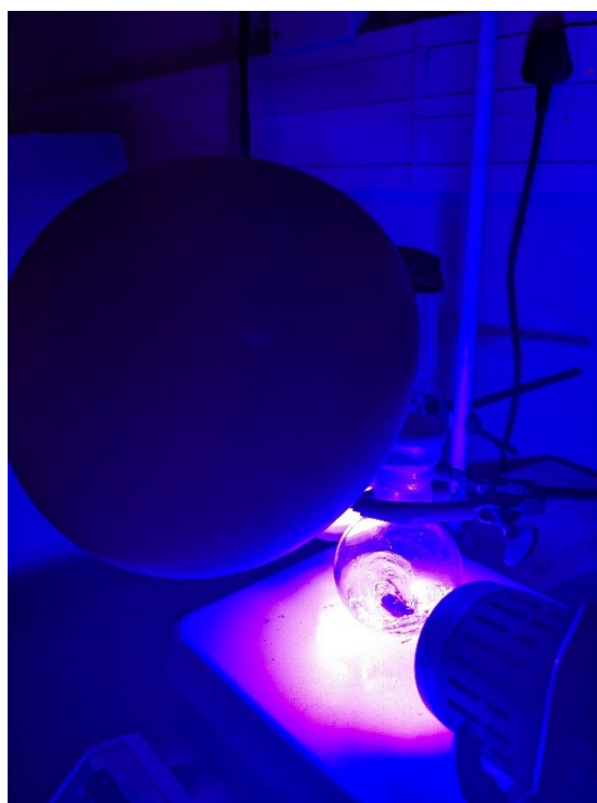
Figure S6. Photoreaction setup for large-scale synthesis. The reaction was performed using Kessil PR160-427 nm lights with 100% light intensity; the distance from the light source to the irradiation vessel is 4 cm.
