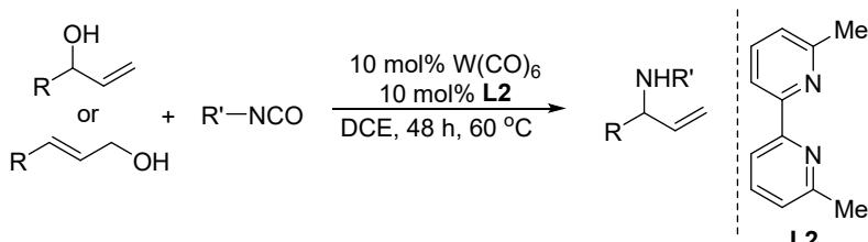
A pressure tube equipped with a magnetic stir bar was charged with W(CO)<sub>6</sub> (10 mol%), **L2** (10 mol%). The tube was purged with argon for 3 minutes. DCE (2 mL) was added followed by the corresponding allylic alcohol (0.6 mmol, 1.5 equiv.) and isocyanate (0.4 mmol, 1.0 equiv.). The tube was sealed with a PTFE lined cap and was stirred in an oil bath at 60 °C for 48 hours. After cooled down, the crude reaction mixture was directly subjected to flash column chromatography.
