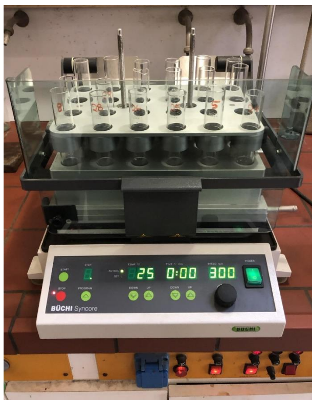
Scheme 1: BUCHI Syncore apparatus utilised for the parallel Knoevenagel reactions.
