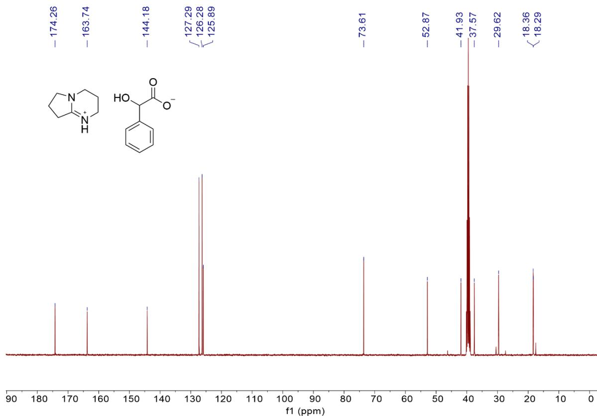
Figure S10. <sup>13</sup>C NMR Spectrum of [DBNH][MAc] (101 MHz, DMSO-d<sub>6</sub>)
