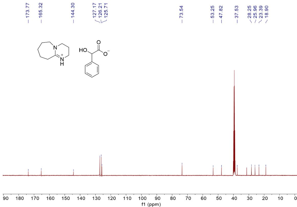
Figure S6.  $^{13}\text{C}$  NMR Spectrum of [DBUH][MAC] (101 MHz,  $\text{DMSO-}d_6$ )
