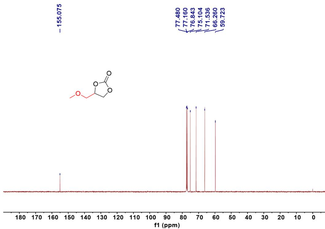
Figure S26. <sup>13</sup>C NMR Spectrum of 4-(methoxymethyl)-1,3-dioxolan-2-one (101 MHz, CDCl<sub>3</sub>)
