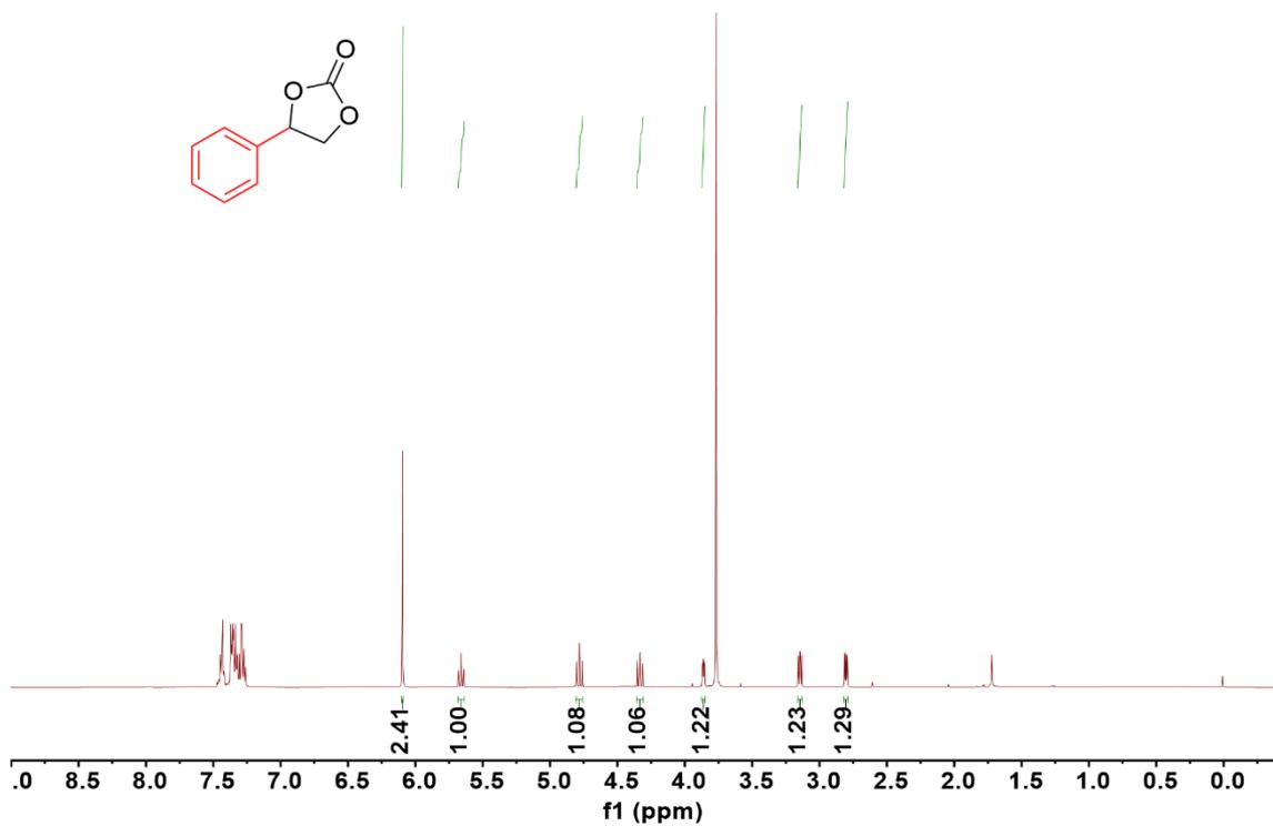
Figure S44.  $^1\text{H}$  NMR Spectrum of 4-phenyl-1,3-dioxolan-2-one (400 MHz,  $\text{CDCl}_3$ ) [DBUH][ALc]
