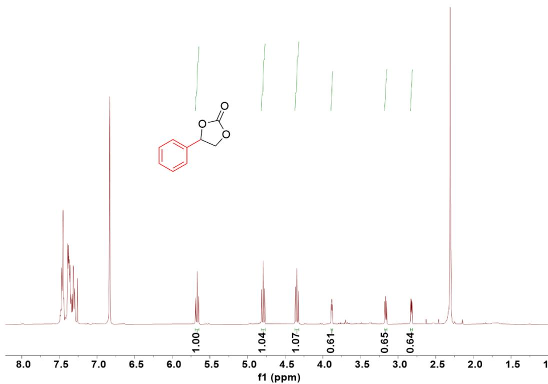
Figure S40.  $^1\text{H}$  NMR Spectrum of 4-phenyl-1,3-dioxolan-2-one (400 MHz,  $\text{CDCl}_3$ ) [DBUH][PAC]
