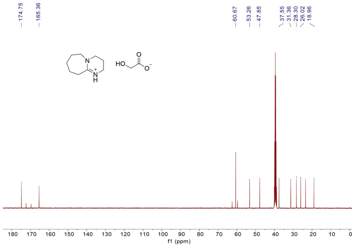
Figure S2.  $^{13}\text{C}$  NMR Spectrum of [DBUH][GAc] (101 MHz,  $\text{DMSO-}d_6$ )
