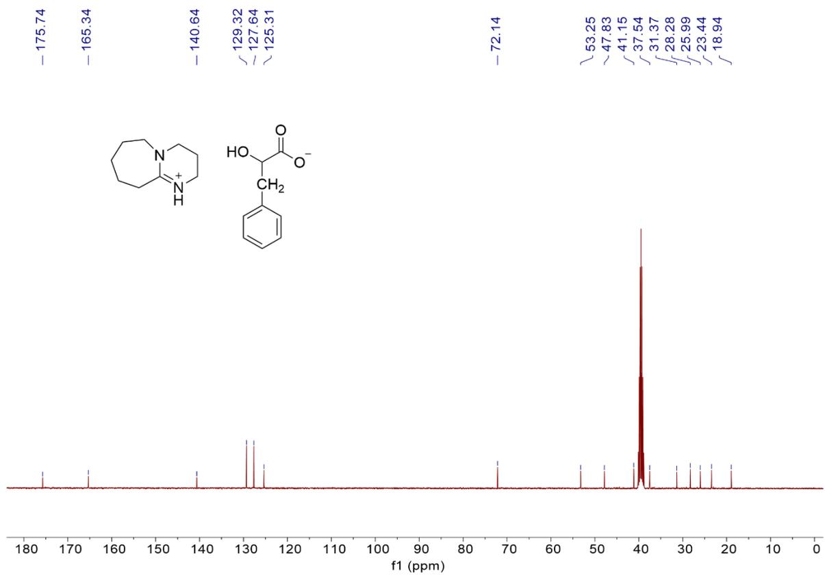
Figure S8. <sup>13</sup>C NMR Spectrum of [DBUH][PLAc] (101 MHz, DMSO-*d*<sub>6</sub>)
