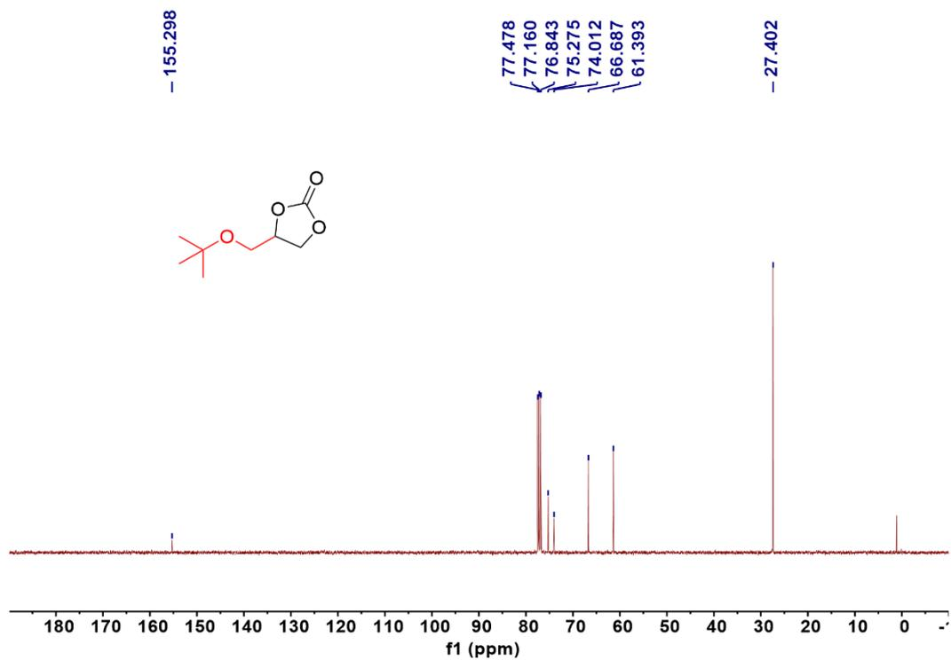
Figure S30. <sup>13</sup>C NMR Spectrum of 4-(*tert*-butoxymethyl)-1,3-dioxolan-2-one (101 MHz, CDCl<sub>3</sub>)
