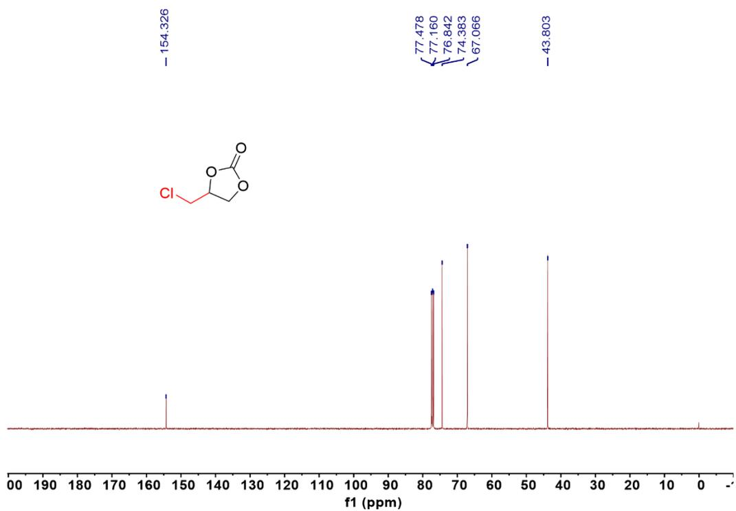
Figure S16.  $^{13}\text{C}$  NMR Spectrum of 4-(chloromethyl)-1,3-dioxolan-2-one (101 MHz,  $\text{CDCl}_3$ )
