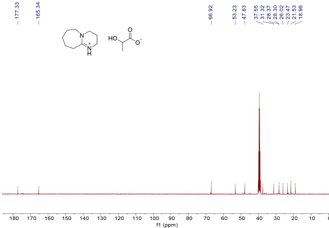
Figure S4.  $^{13}\text{C}$  NMR Spectrum of [DBUH][Lac] (101 MHz,  $\text{DMSO-d}_6$ )
