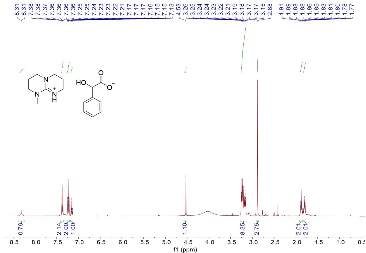
Figure S11. <sup>1</sup>H NMR Spectrum of [MTBDH][MAc] (400 MHz, DMSO-d<sub>6</sub>)
