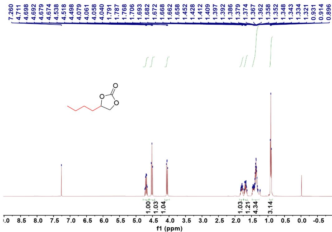
Figure S23.  $^1\text{H}$  NMR Spectrum of 4-butyl-1,3-dioxolan-2-one (400 MHz,  $\text{CDCl}_3$ )
