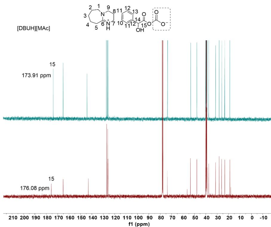
Figure S38.  $^{13}\text{C}$  spectra (DMSO- $d_6$ ) of [DBUH][MAc] during the absorption of  $\text{CO}_2$  (b), Pure [DBUH][MAc] (a),  $\text{CO}_2$  (1 Mpa), Catalyst[DBUH][MAc]
