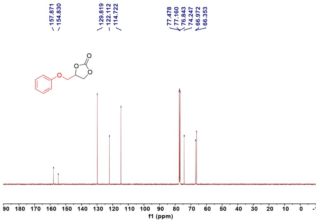
Figure S32. <sup>13</sup>C NMR Spectrum of 4-(phenoxymethyl)-1,3-dioxolan-2-one (101 MHz, CDCl<sub>3</sub>)
