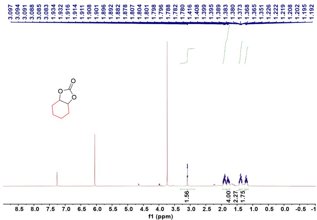
Figure S35. <sup>1</sup>H NMR Spectrum of hexahydrobenzo[d]-1,3-dioxolan-2-one (400 MHz, CDCl<sub>3</sub>)
