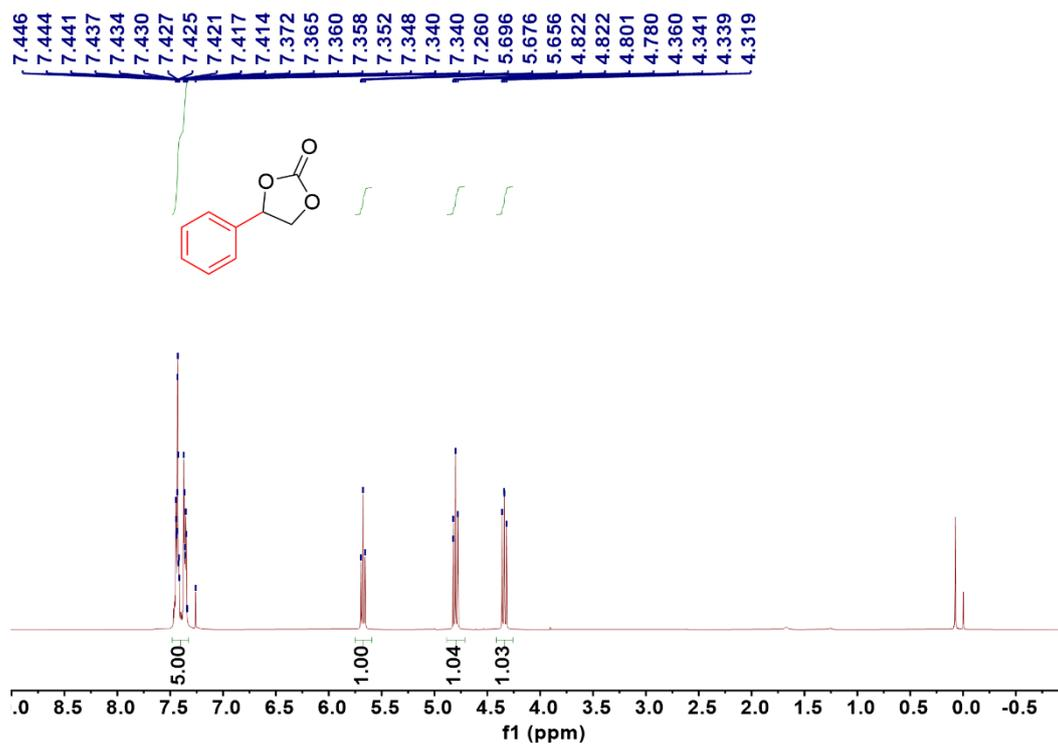
Figure S33. <sup>1</sup>H NMR Spectrum of 4-phenyl-1,3-dioxolan-2-one (400 MHz, CDCl<sub>3</sub>)
