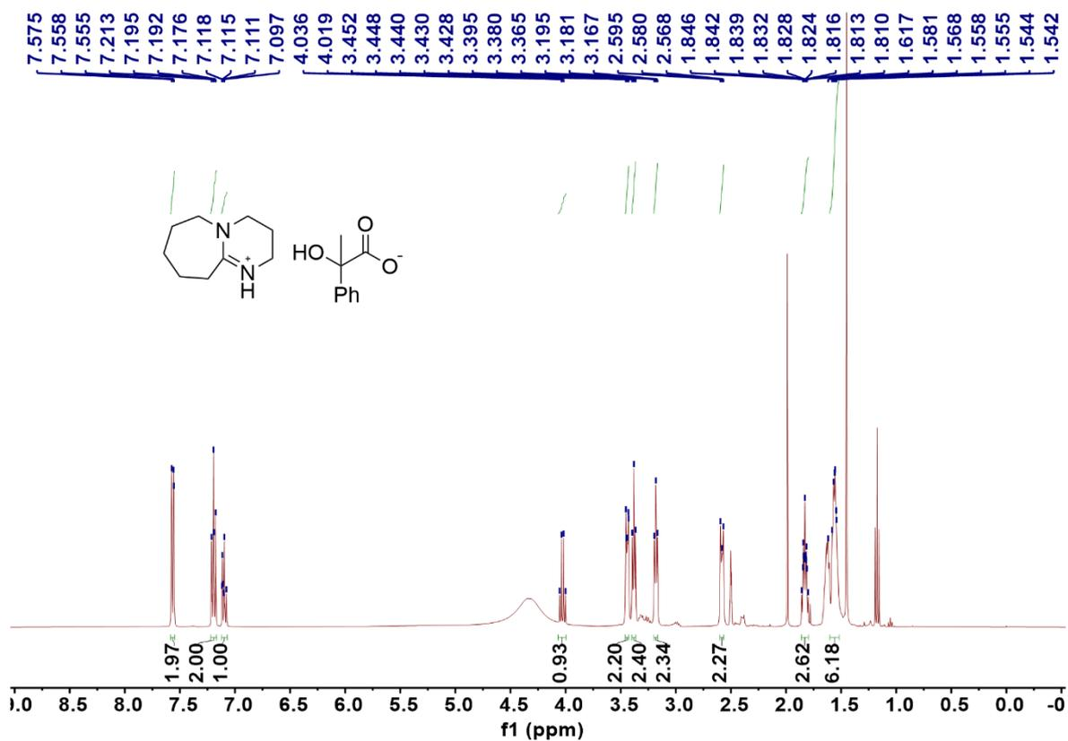
Figure S43.  $^1\text{H}$  NMR Spectrum of [DBUH][ALc] (400 MHz,  $\text{DMSO-}d_6$ )
