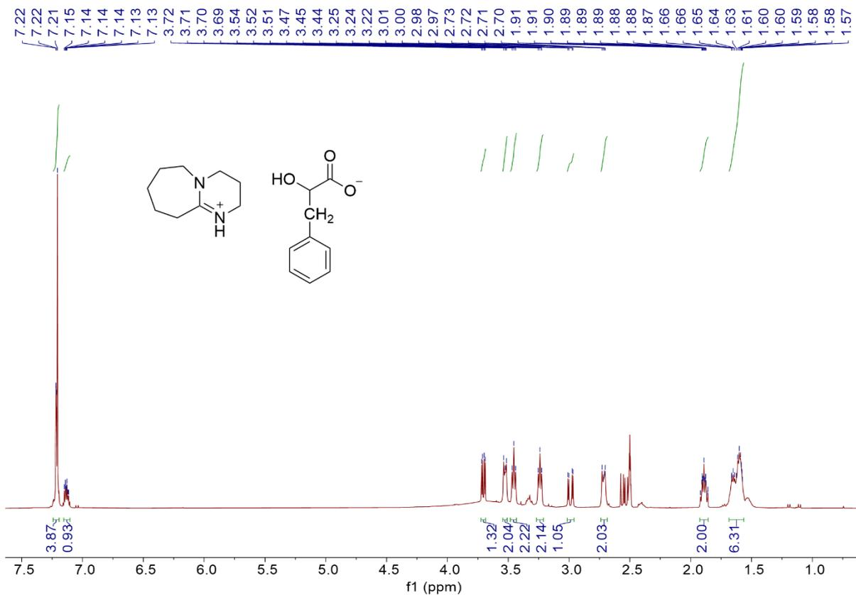
Figure S7.  $^1\text{H}$  NMR Spectrum of [DBUH][PLAc] (400 MHz,  $\text{DMSO-}d_6$ )
