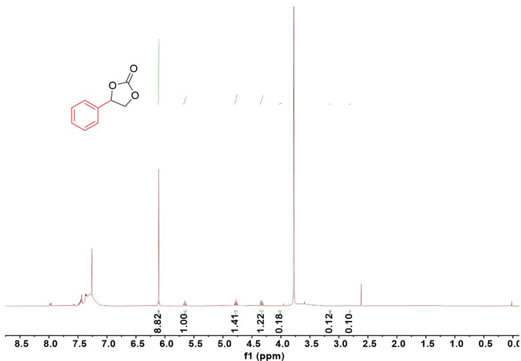
Figure S45. <sup>1</sup>H NMR Spectrum of 4-phenyl-1,3-dioxolan-2-one (400 MHz, CDCl<sub>3</sub>) [DBUH][MAc]
