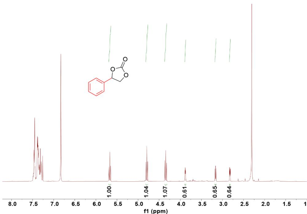
Figure S37.  $^1\text{H}$  NMR Spectrum of 4-phenyl-1,3-dioxolan-2-one (400 MHz,  $\text{CDCl}_3$ ) catalyst:[DBUH][Pac]
