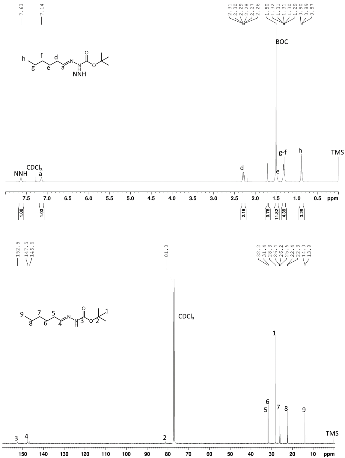
Figure S58. The 400MHz ^1\text{H} and 100 MHz ^{13}\text{C} NMR Spectra of tert -butyl 2-hexylhydrazonocarboxylate in \text{CDCl}_3 .
