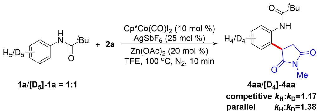
**Intermolecular competition KIE experiment.** Amide **1a** (35.5 mg, 0.2 mmol), **[D<sub>5</sub>]-1a** (36.4 mg, 0.2 mmol), maleimide **2a** (66.7 mg, 0.6 mmol),  $\text{Cp}^*\text{Co}(\text{CO})\text{I}_2$  (19.0 mg, 0.04 mmol),  $\text{AgSbF}_6$  (34.2 mg, 0.10 mmol),  $\text{Zn}(\text{OAc})_2$  (14.6 mg, 0.08 mmol) and TFE (2.0 mL) were added to a 35 mL Schlenk flask equipped with a high-vacuum PTFE valve-to-glass seal. Then the flask was sealed under  $\text{N}_2$  and stirred at 100 °C for
