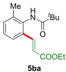
Ethyl (*E*)-3-(3-methyl-2-pivalamidophenyl)acrylate (**5ba**)<sup>5</sup>. Purification by column chromatography on silica gel (eluent: petroleum ether:ethyl acetate=8:1, v/v) afforded **5ba** as a white solid (23.1 mg, 40% yield); mp 92-94 °C;  $R_f = 0.5$  (petroleum
