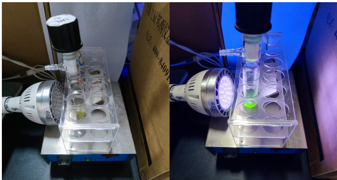
Figure S1. Photoreactor used in this work (45 W purple LEDs, \lambda_{\text{max}} = 395 \text{ nm} ).
