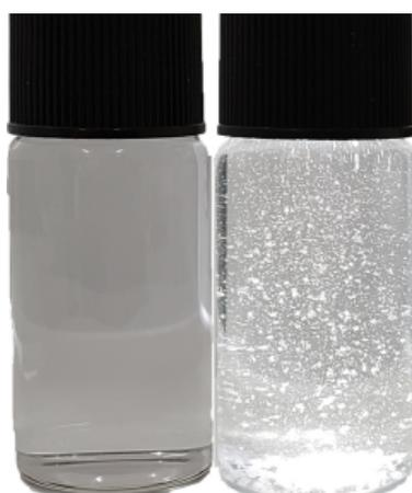
**Figure S2** Photographic demonstration of the dissolution cases involving 0.1 g of ammonium persulfate in 10 mL of water (left) and ethylene glycol (right).
