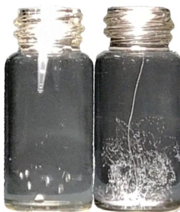
**Figure S3** Photographic demonstration of the droplets of neat EDOT and EDOT/EG mixture (v/v 1/5) in water.
