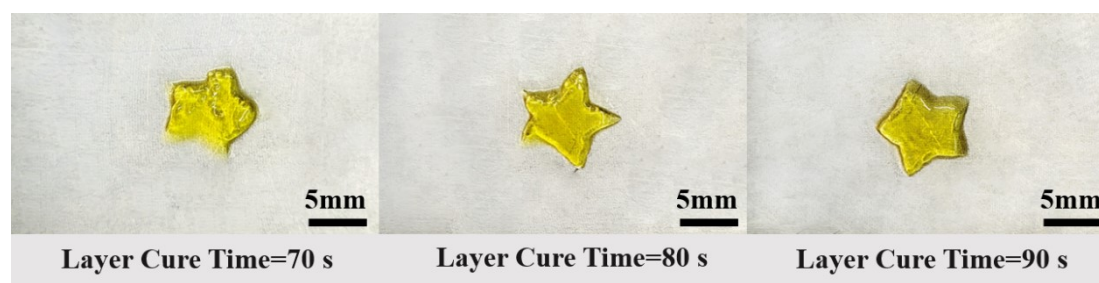
Figure S9. 3D printing resolution comparison for hydrogel when changing the layer cure time (Layer Thickness=300 \mu\text{m} ).
