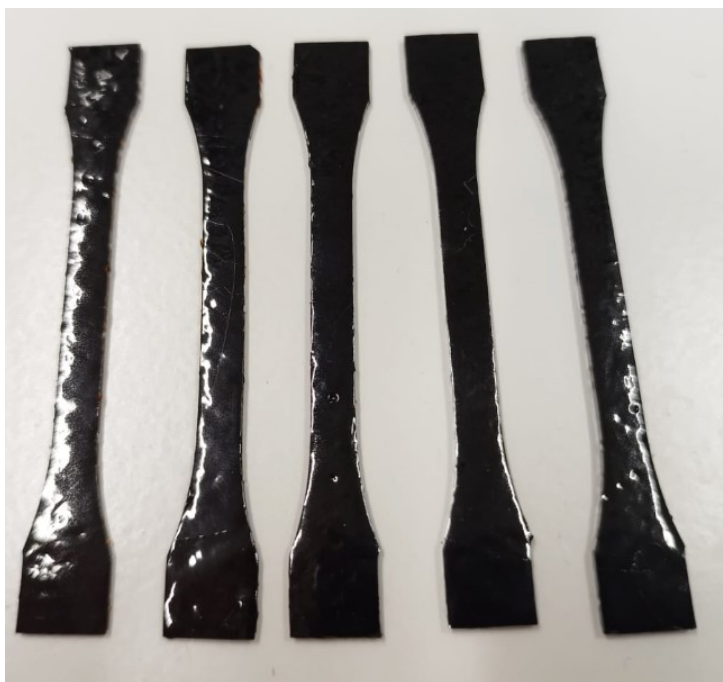
Figure 1: Example of test specimens used for cyclic mechanical tests and tensile testing
