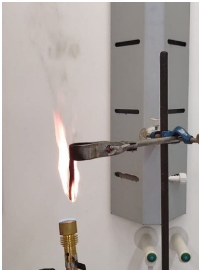
Figure 3: Impression of soot-evolution and flame during burn test.
