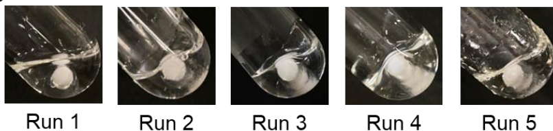
Figure S2. Appearance of polymerized products obtained by free radical polymerization of NIPAM in various NADESs (see Table 1 and Table S2 for detailed polymerization conditions).
