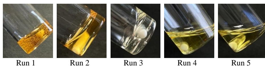
Figure S9. Appearance of polymerized products obtained by photo-induced free radical polymerization of NIPAM in various NADESs (see Table S6).
