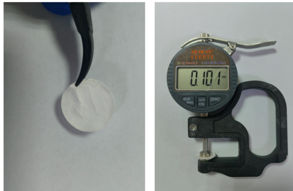
Fig. S1. Optical images of PVDF-HFP nanofiber membrane and the measurement of the thickness.
