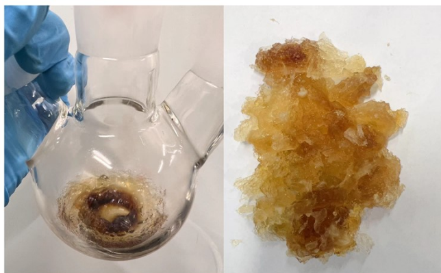
Figure S3. Severe cross-linking of PIC occurred when isosorbide contained 1.5 mol% 2-deoxy-D-ribose impurity, as well as a gel produced by solubilization in \text{CHCl}_3 .
