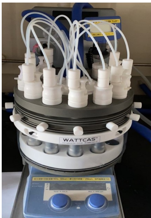
Fig. S9 WP-TEC-1020HSL photochemical reaction system.
