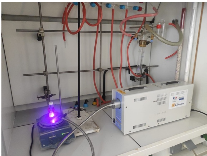
Fig. S2. Experimental setup of SFEP of GlyMA at room temperature under 405 nm (30 mW) irradiation using a light source (Opto-Spectrum Generator L12194-00-39-070).
