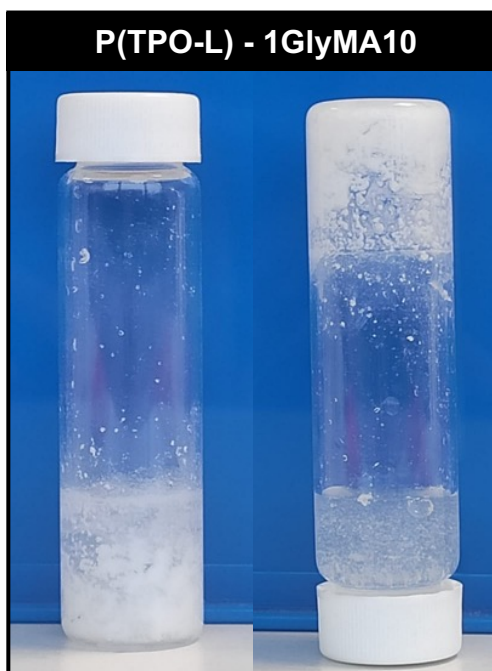
Fig. S8. Surfactant-free latex prepared via SFEP of GlyMA at RT SC=10% w/w and R=1 ‰ in water using TPO-L under 405 nm (P(TPO-L)-1GlyMA10).
