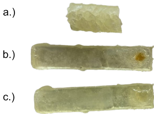
Figure 1 SI frontally polymerized a.) reference sample; b.) PH20 sample; c.) SH20 sample
