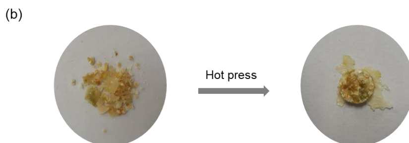
Fig. S13. (a) Synthesis of polyurea vitrimer PUA8-S . (b) Failure of reprocessing for PUA8-S .
