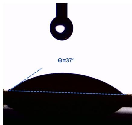
**Fig. S8.** The water contact angle of Salen-TAPT-COF/PP.
