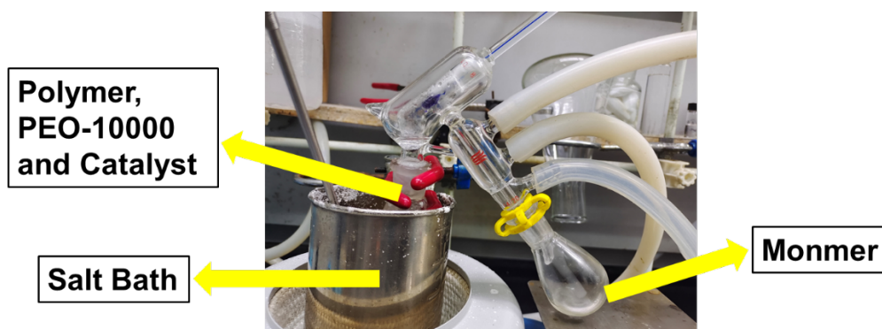
Fig. S22 Thermal depolymerization of polymer to monomer via vacuum distillation.
