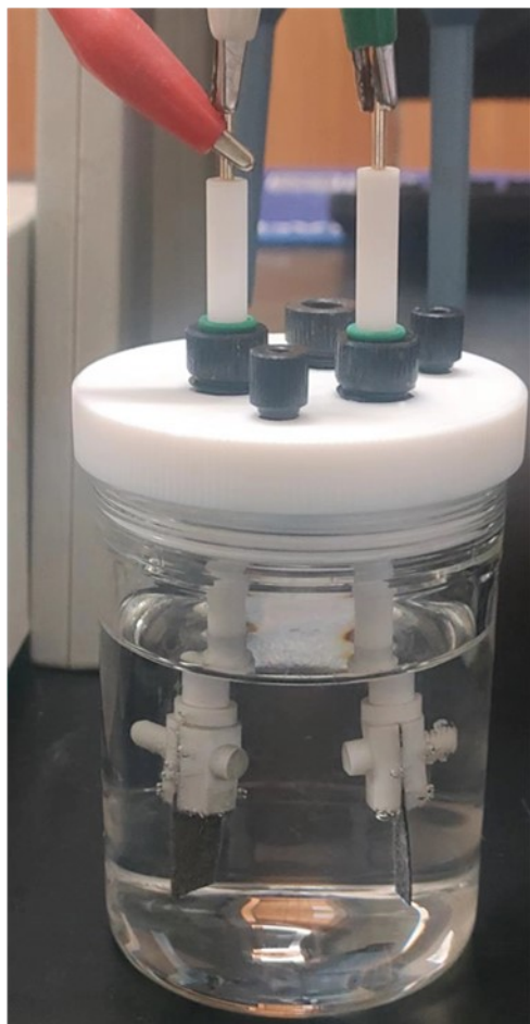
Fig. S12 (a) Optical picture of the water-splitting device. (b) Optical pictures of the electrodeposition samples.
