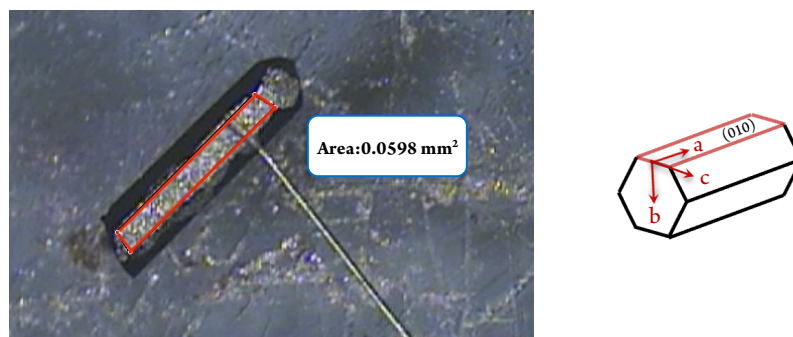
Figure S11. The pyroelectric measurement was carried out as a previously reported method. 6-8 The single crystal for pyroelectric measurement (Left). The index of crystal (Right). To ensure the pyroelectric current could be detected by our electrometer, the area of plane (010) should be at least 0.04 mm 2 .
