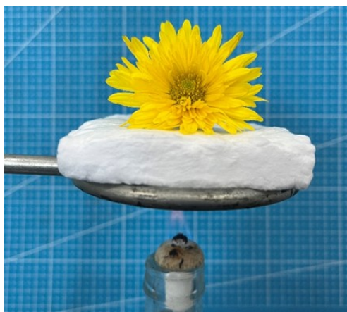
Figure S18 The thermal insulation of \text{ZrO}_2 @Mullite nanofibrous aerogels
