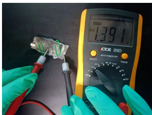
Fig. S19. Open circuit voltage of solid-state ZAB tested by a universal meter.
