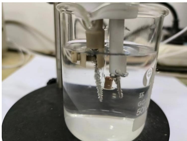
Fig. S6 An electrolytic cell with close electrode spacing.
