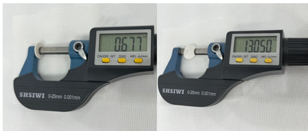
Fig. S17. The P-TT pellet was obtained by the classic powder's pressing method (18 MPa).
